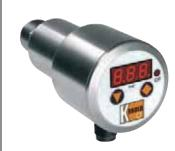
Measuring range: -30 ... 0" Hg through 0 ... 5,800 PSIG Display: 3-digit LED Power supply: 24 V<sub>DC</sub> Connection: 1/4", 1/2" NPT Accuracy: ± 0.5 - 1 % of full scale
