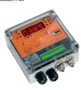
Measuring range: 0 ... 20" H<sub>2</sub>O Power supply: 24 V<sub>AC/DC</sub>, 110 V<sub>AC</sub>, 230 V<sub>AC</sub> Display: 4-digit LED Connection: 1/4" tube Accuracy: ± 1.6 % of full scale
