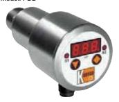
Measuring range:  $-30^{\circ} \dots 0^{\circ} \text{ Hg through } 0 \dots 5,800 \text{ PSIG}$  Display: 3-digit LED Power supply:  $24 \text{ V}_{DC}$  Connection: \$%'\$, \$%'\$ NPT Accuracy:  $\pm 0.5 - 1 \text{ $\%'$} \text{ full scale}$
