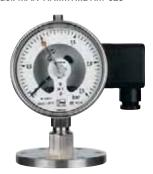
Measuring range: 0 ... 15 PSIG through 0 ... 580 PSIG Housing: Ø 100, 160 mm Connection: 1" to 4" ANSI Accuracy: ± 1.6 % of full scale
