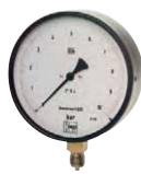
Measuring range: -8.5" ... 0" Hg ... 0 ... 36,000 PSIG Housing: Ø 160, 250 mm Overload protection: 1,0 times Connection: 1/2" NPT Accuracy: ± 0.25 or ± 0,6 % of full scale
