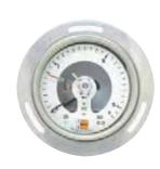
Measuring range: -30" ... 0" Hg through 0 ... 23,000 PSIG Housing: Ø 100, 160 mm Overload protection: 1.15-1.3 times Connection: ½" NPT Accuracy: ± 1.0 of full scale
