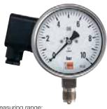
Measuring range: -30" ... 0" Hg through 0 ... 8,700 PSIG Housing: Ø 100 Overload protection: 0.9-1.0 times Connection: ½" NPT 2-wire 4-20 mA output Accuracy: ± 1.0 of full scale
