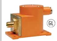
Measuring range: -30 ... 0" Hg through 0 ... 1,450 PSIG Overload protection: 1,6 times Connection: M16x1,5 (NPT with adapter) Accuracy: ± 1 % of full scale
